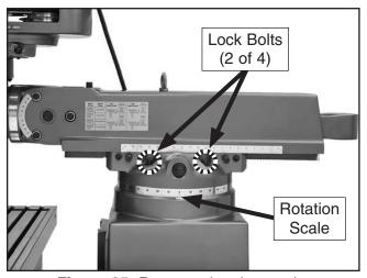
Figure 25. Ram rotational controls.
